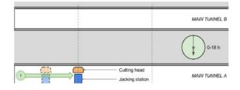
Stage 1: Positioning of jacking station and cutting head.
