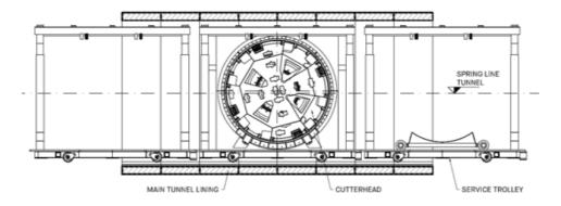
Fig. 19 - General features of cutter head (Courtesy: SWS Global Engineering, 2016)
