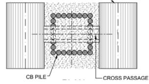
Fig.12 - Typical plan of a top down excavation method
