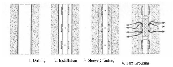
Fig. 4 -TAM grouting schematic (Courtesy: Spargrp.com)
