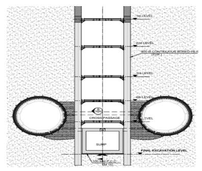
Fig. 14 - Installation of struts for excavation
