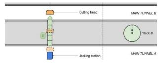
Stage 2:Exacavation and construction of first cross passage
