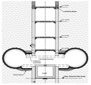
Fig. 15 -Cutting of CB pile at CP level
