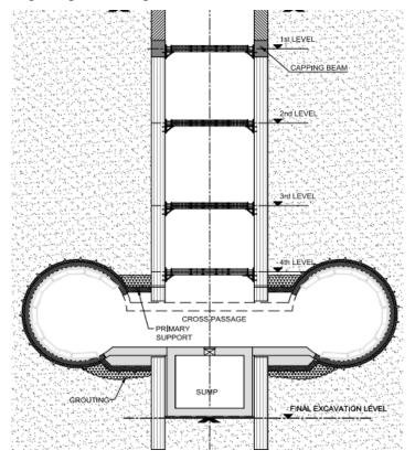
Fig. 16 - Casting of base slab and CP walls
