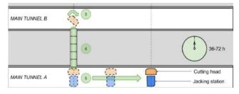
Stage 3: Cutting head retrieval and reassembly
