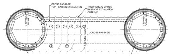
Fig. 1 - Typical excavation scheme
