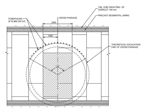
Fig. 3 - Pipe roofing (on the cross passage face)
