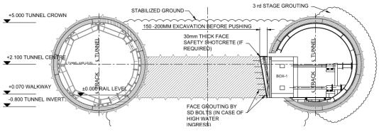
Fig. 11 - Excavation scheme of cross passage
