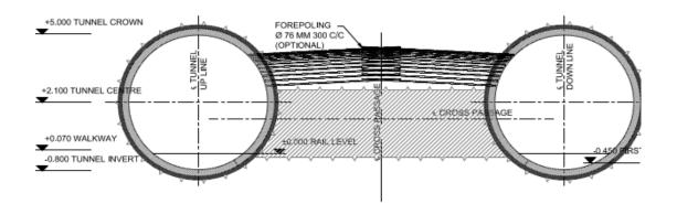
Fig. 2 - Pipe roofing scheme (L-Section)
