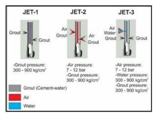
Fig.6 - Types of jet grouting
