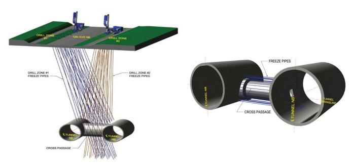
Fig.8 - Typical vertical and horizontal ground freezing scheme (Sopko et al., 2013)
