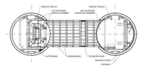
Fig.18 - Typical arrangement for cross passage excavation through TBM
