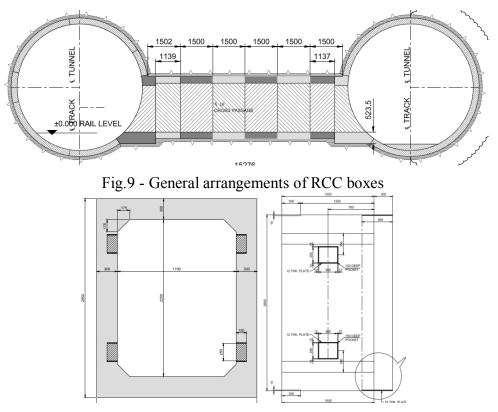
Fig.10 - Cross section and longitudinal section of RCC box
