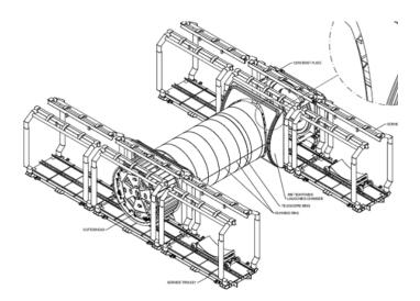
Fig. 17 - Isometric view of small scale secondary TBM (Courtesy: SWS Global Engineering, 2016)
