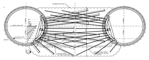
Fig. 5 - TAM grouting in cross passages
