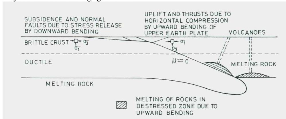
Fig. 2 - State of stresses in colliding inter-plate boundaries
