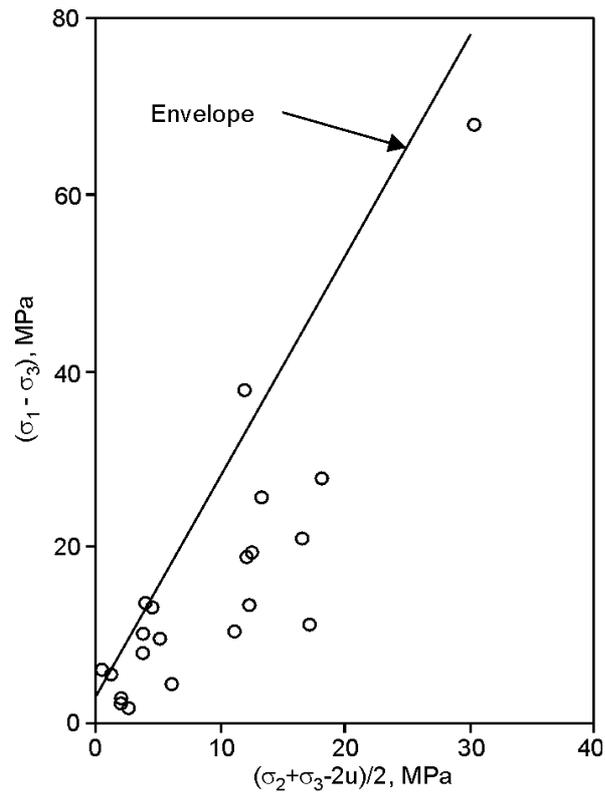
Fig. 3- Plot of in-situ stresses showing upper bound
