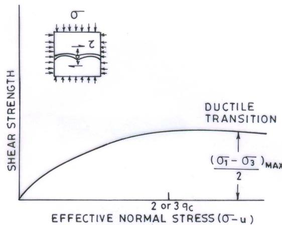
Fig.1 - Shear strength of discontinuities at very high confining stress (Barton, 1976)
