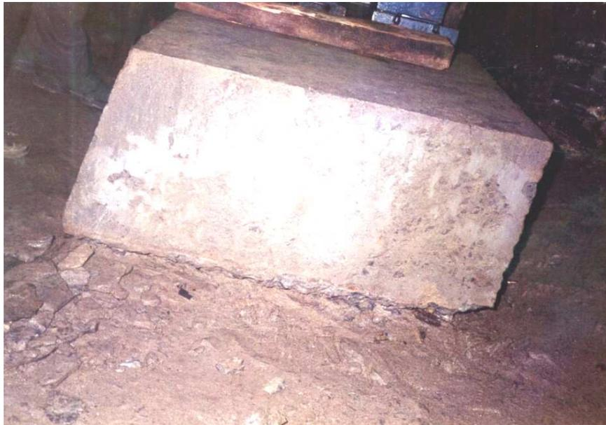
Fig. 5 - Shear test block after shearing
