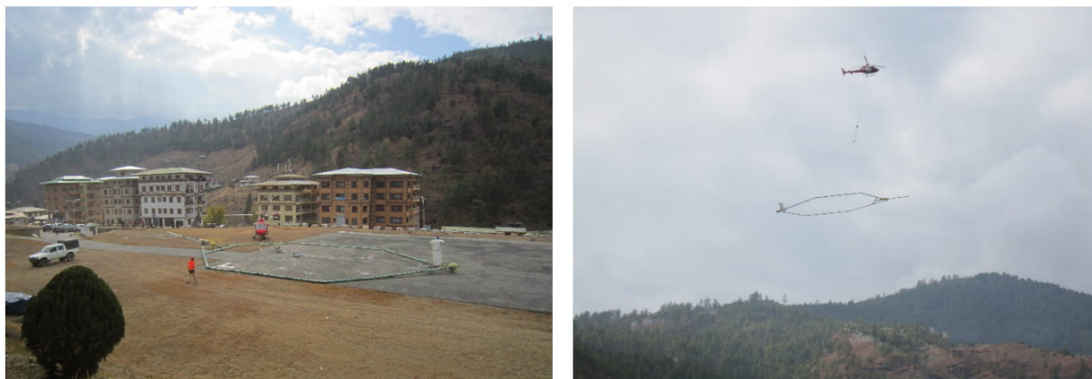
Fig. 6 - Preparation for AEM survey (left) and performing AEM survey along tunnel alignment
