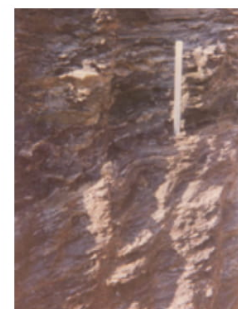
Fig. 16: Moderately good granite gneiss rock strata at EL 518m
