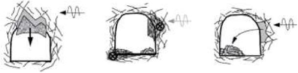
Seismically induced fall Rock fracture with dilation Block ejection Fig. 3 - Rock burst damage mechanisms (Kaiser et al., 1996)
