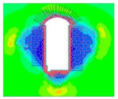
Fig. 6 - Rock mass damaged zone (shown by small circles for shear failure and cross for tension failure) around the cavern (Bhasin and Pabst, 2014)
