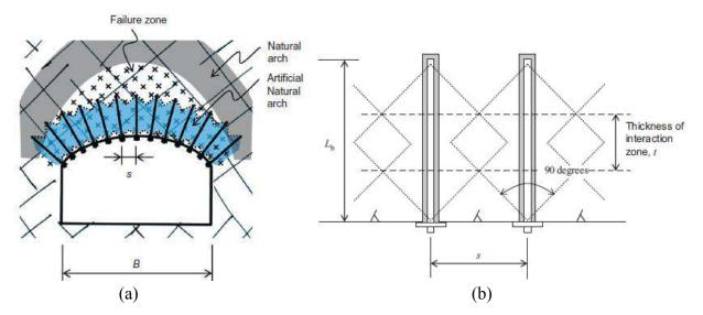
Fig. 5 - (a) Stablishing of artificial arch above the tunnel with rock reinforcement and (b) Reinforcement mechanism of rock mass (Li, 2017)
