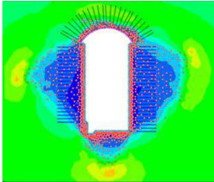
Fig. 6 - Rock mass damaged zone (shown by small circles for shear failure and cross for tension failure) around the cavern (Bhasin and Pabst, 2014)
