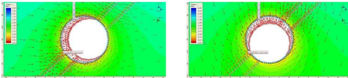
Fig. 2- Effect of two parallel joints in competent rock during static & seismic loading. Note how the joints act as waveguides and stress collectors (right figures) when seismic loading is applied (Bhasin and Pabst, 2014)
