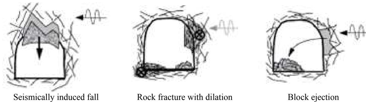
Fig. 3 - Rock burst damage mechanisms (Kaiser et al., 1996)
