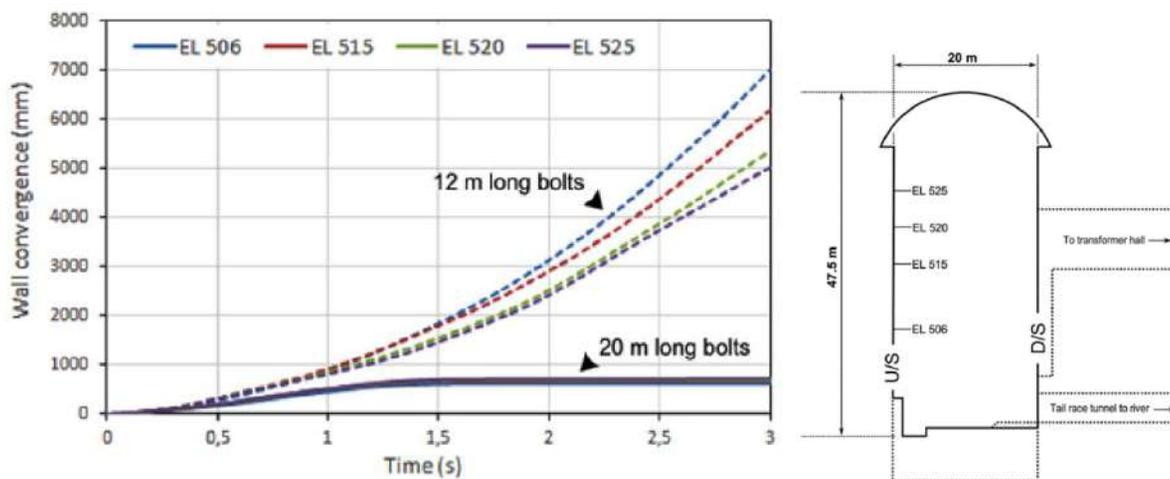
Fig. 7 - Convergence of walls of the cavern with time obtained by dynamic analysis (Bhasin and Pabst, 2014)
