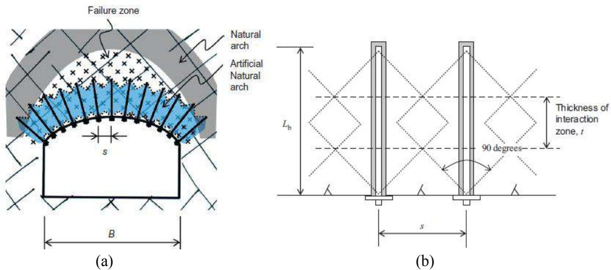
Fig. 5 - (a) Stabliishing of artificial arch above the tunnel with rock reinforcement and (b) Reinforcement mechanism of rock mass (Li, 2017)
