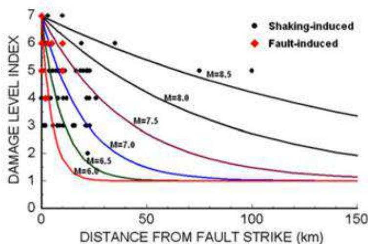
Fig. 1 - Relation between distance from surface trace of the fault and damage level index (DLI) (Aydan et al., 2010)
