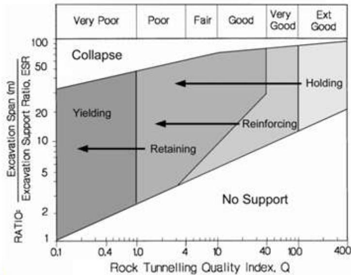
Fig. 4 - Rock support functions in the stability graph of Q-System (Kaiser et al., 2000)
