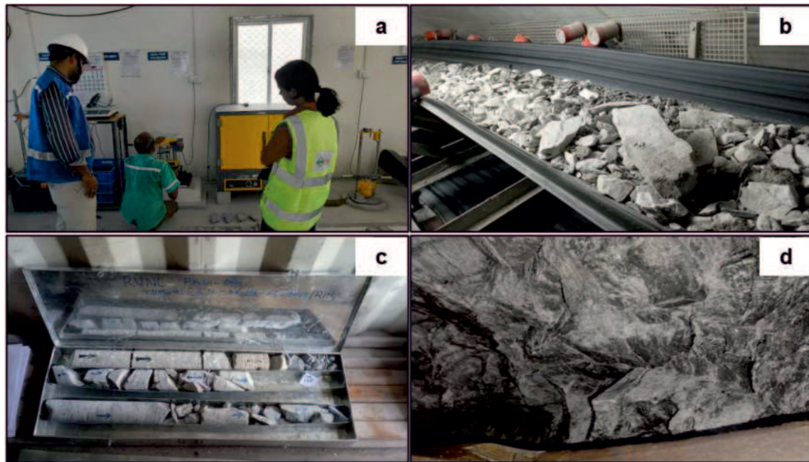
Figure 3 - Geological and geotechnical investigations during TBM operation, (a) point load test (b) muck assessment during mining (c) rock core drilling and logging (d) face mapping
