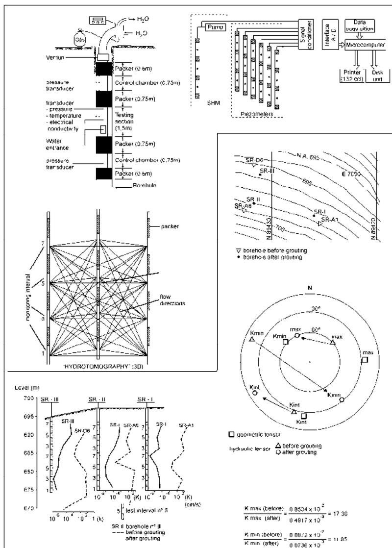
Fig. 11 - Three-dimensional permeability testing performed between three boreholes, both before and after grouting, showed rotation and reduction of permeability tensors, and greatly increased bulk modulus. Despite use of industrial cement and bentonite, the permeable rock mass was greatly improved. Quadros et al. (1995)
