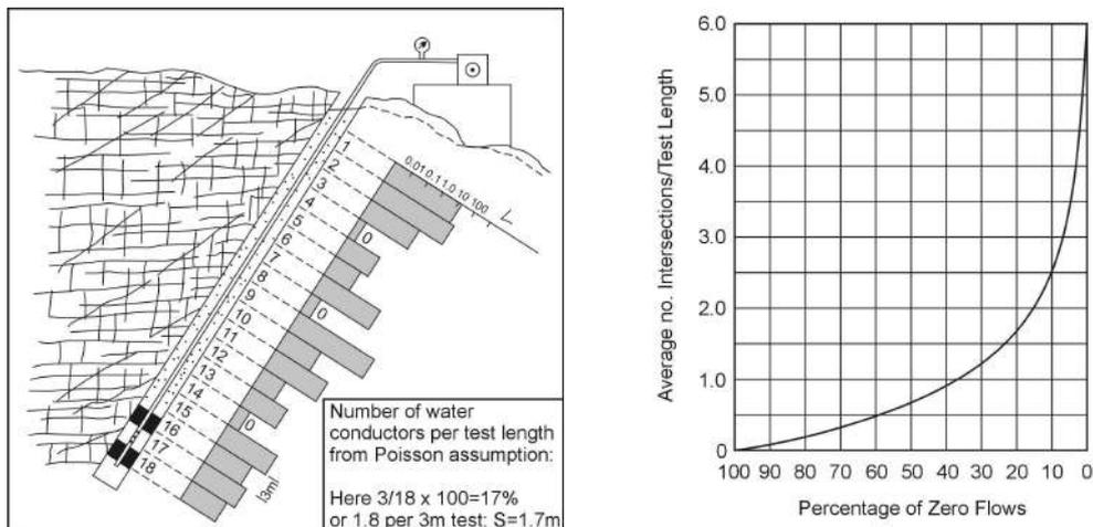
Fig. 3 - Left: Lugeon testing and zero flow sections as a percentage of the total. Right: Poisson distribution for interpreting average number of water conductors. (17% zeros: 1.8 conductors/test length:  $S=1.7\text{m}$ ). Snow (1968).
