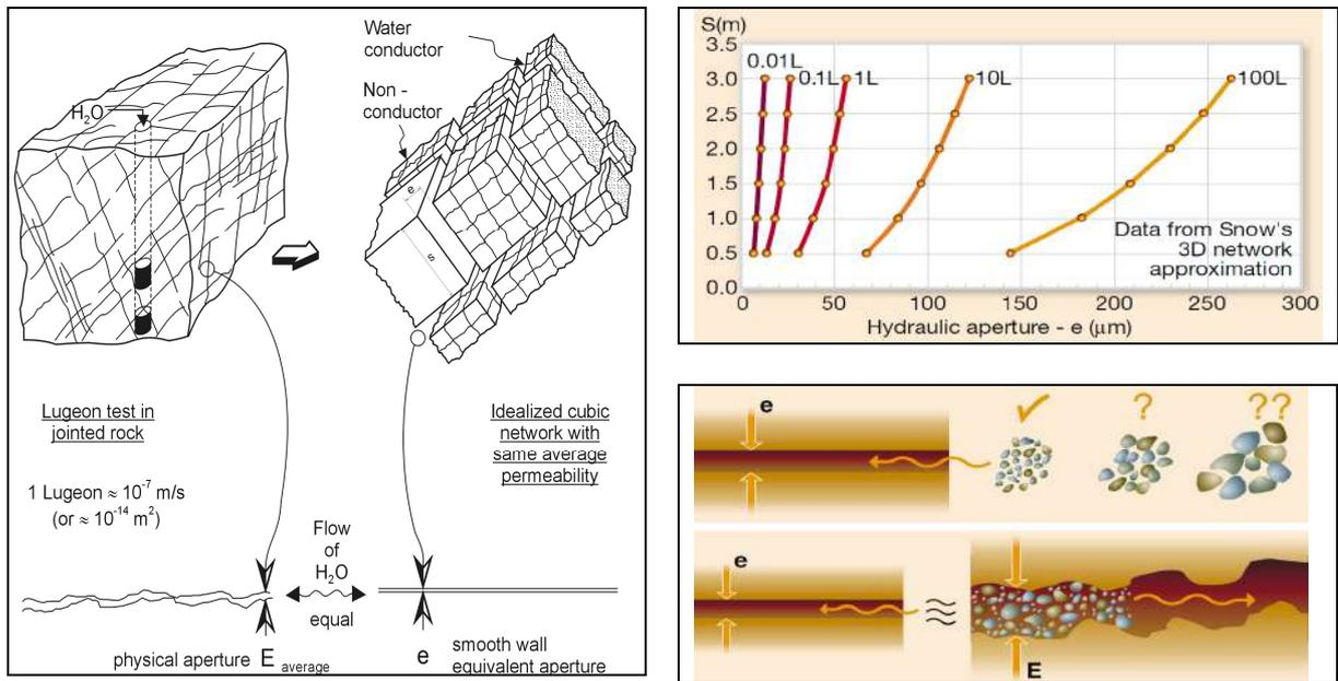
Fig. 4 - Left: Representing a regularly-jointed rockmass with a cubic network of hydraulic conductors of mean aperture (e) and mean spacing (S), based on Snow (1968). Right: Estimates of (e) and (S) from equation 3, and the aperture inequality  $E \geq e$ , which allows grout particles to penetrate real joints (E) even when (theoretical) hydraulic apertures (e) are apparently too small.
