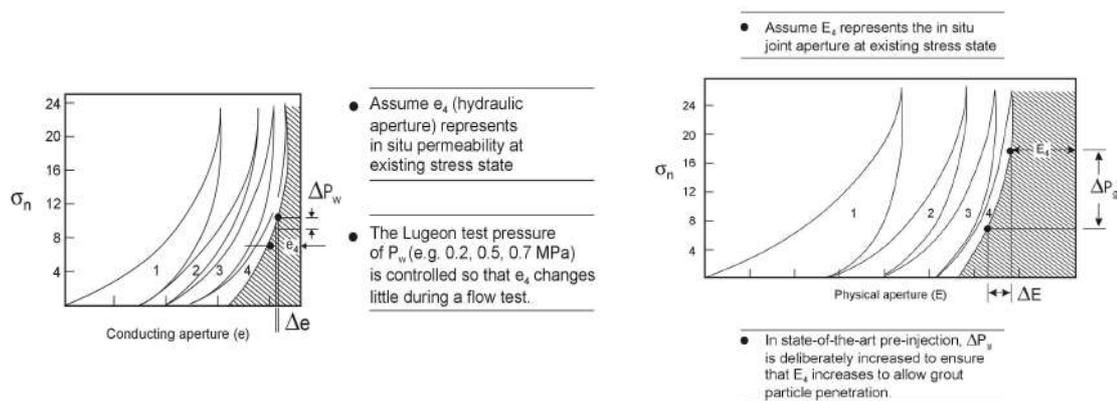
Fig. 8 - The secret of successful pre-grouting, besides grout particle technology improvements, such as use of micro-silica, is to make  $\Delta P_g \gg \Delta P_w$ , so that  $\Delta E \gg \Delta e$ . (Barton-Bandis joint normal closure/opening model)
