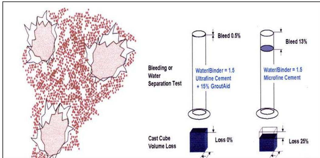
Fig. 10 - Stable non-bleeding, non-shrinking grouts are essential for preventing ‘water-sick’ rock and poor pre-injection results. It is a false ‘economy’ to reject grout additives because of high unit prices. The left drawing contrasts cement particles with micro-silica particles, which are as fine as smoke. (Priv.comm., S. Roald /Elkem)
