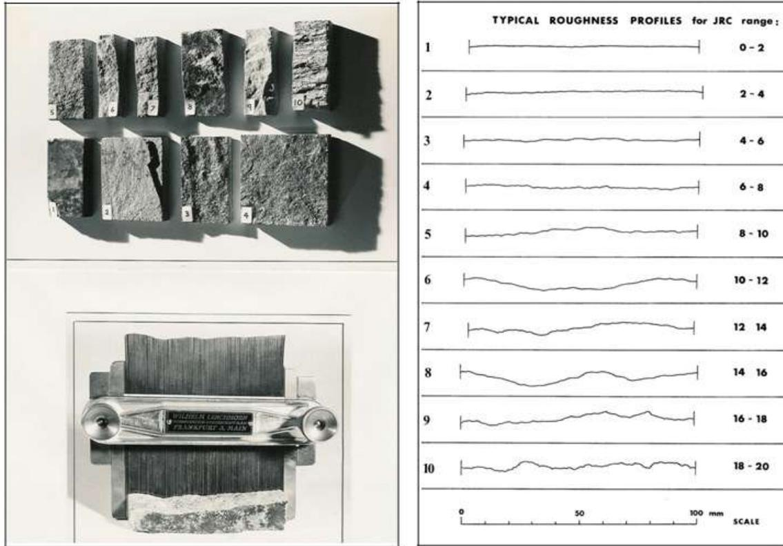
Fig. 6 - Examples of joint surfaces that provided the given ranges of  $JRC_0$  (100 mm scale) roughness. These values of  $JRC_0$  allow an approximate conversion from  $e$  to  $E$  (Barton and Choubey, 1977)
