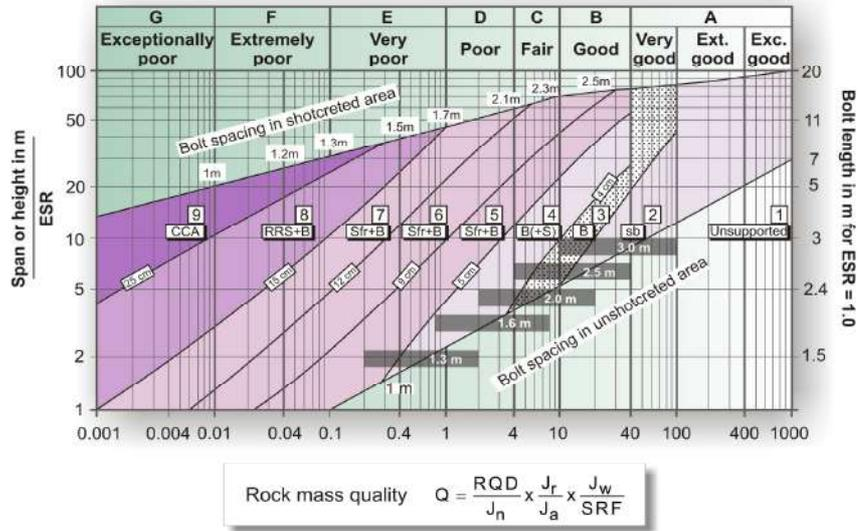
Fig. 13 - Q-system based estimation of permanent support needs for tunnels and caverns, assuming NMT (single-shell) principles for fast economic tunnelling (Grimstad and Barton, 1993)
