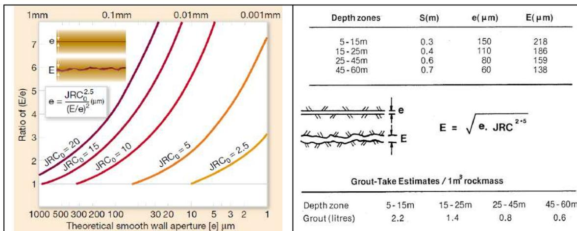
Fig. 5 - Left: The inequality of (E) and (e) for mated joints under normal closure (or opening) is a function of joint roughness coefficient JRC<sub>0</sub>. Right: an example of application of the above methods (e, S, JRC<sub>0</sub> and E), from 1978, at a permeable dam site in Surinam, where joints in the core were roughness-profiled. Barton et al. (1985)
