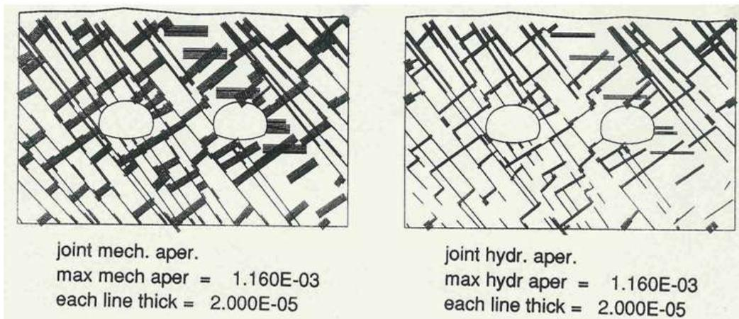
Fig. 7 - Examples of joint apertures  $E$  and  $e$  in an NGI UDEC-BB model of twin tunnels (The maxima are equal due to corner-of-block channel apertures exceeding 1mm) (Pers. comm.. A. Makurat, 1988).
