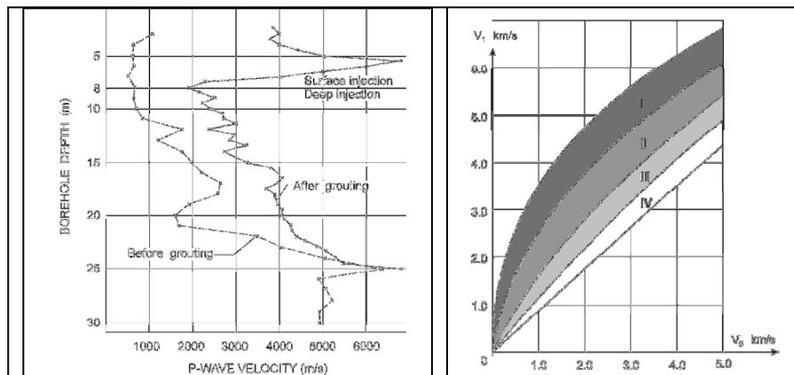
Fig. 14 - Left: Before and after grouting effects on cross-hole velocity at the Norwegian Oddatjørn dam abutment. By (1988). Right: Grouting efficiency (I excellent, II good, III satisfactory, IV unsatisfactory) based on velocity monitoring at the Inguri arch dam (Savich et al., 1983)
