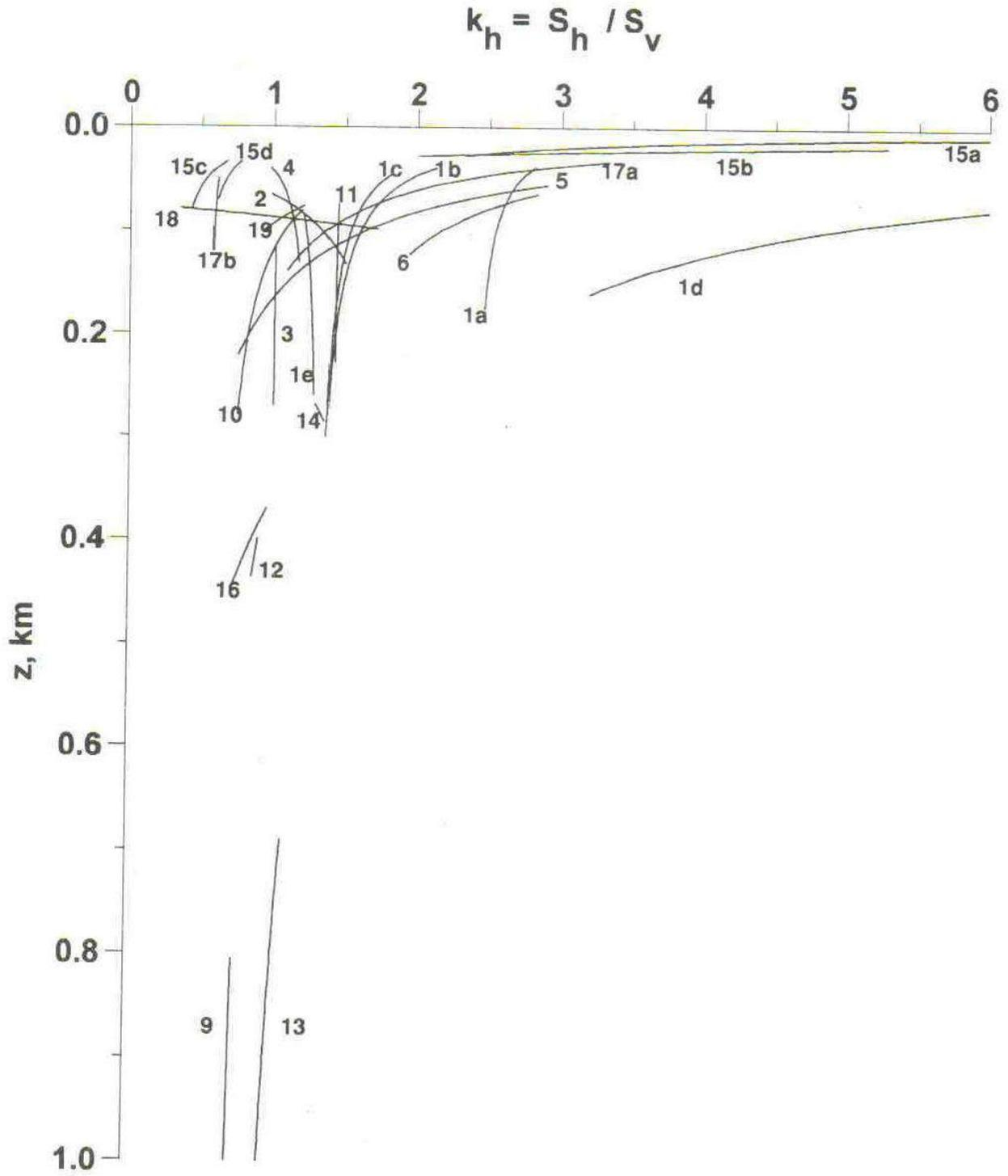
Fig. 4 (b) :  $S_h/S_v$  for about 20 borehole locations in central Germany.
