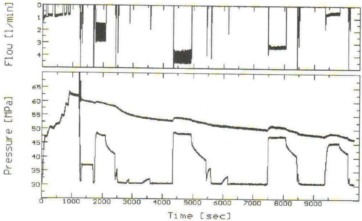
Fig. 2: A hydrofrac pressure and pumping rate record measured in borehole GPK1 of the European Hot Dry Rock Project at Soutz-sous-Forêts at a depth of 3500 m at a temperature of about 150°C and in hostile saline environment.
