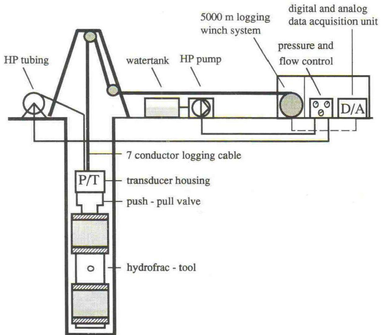
Fig. 1 : Schematic view of the wireline hydrofrac technology.
