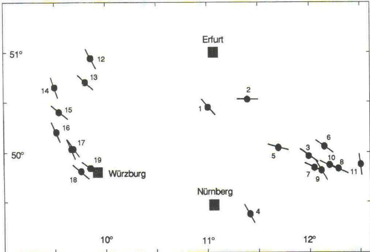
Fig. 3: The orientation of the maximum horizontal stress  $S_H$  at about 20 borehole locations in central Germany.
