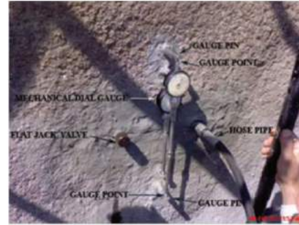
Fig.7: Placing of dial gauge after fixing flat jack between two pins
